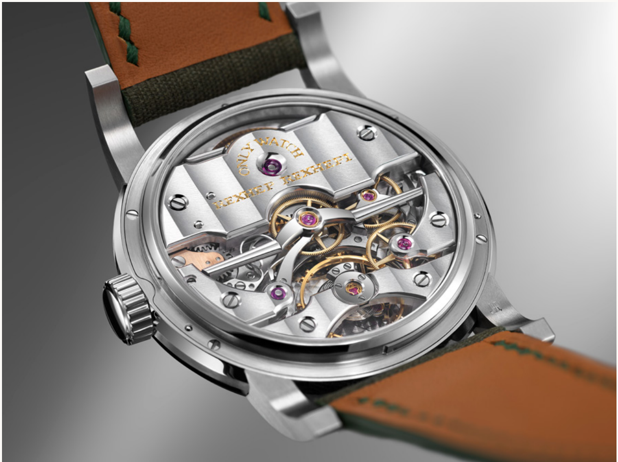
In-house, manually-wound movement. Hours, minutes and central seconds. Hacking, zero-reset seconds for precise time setting.
